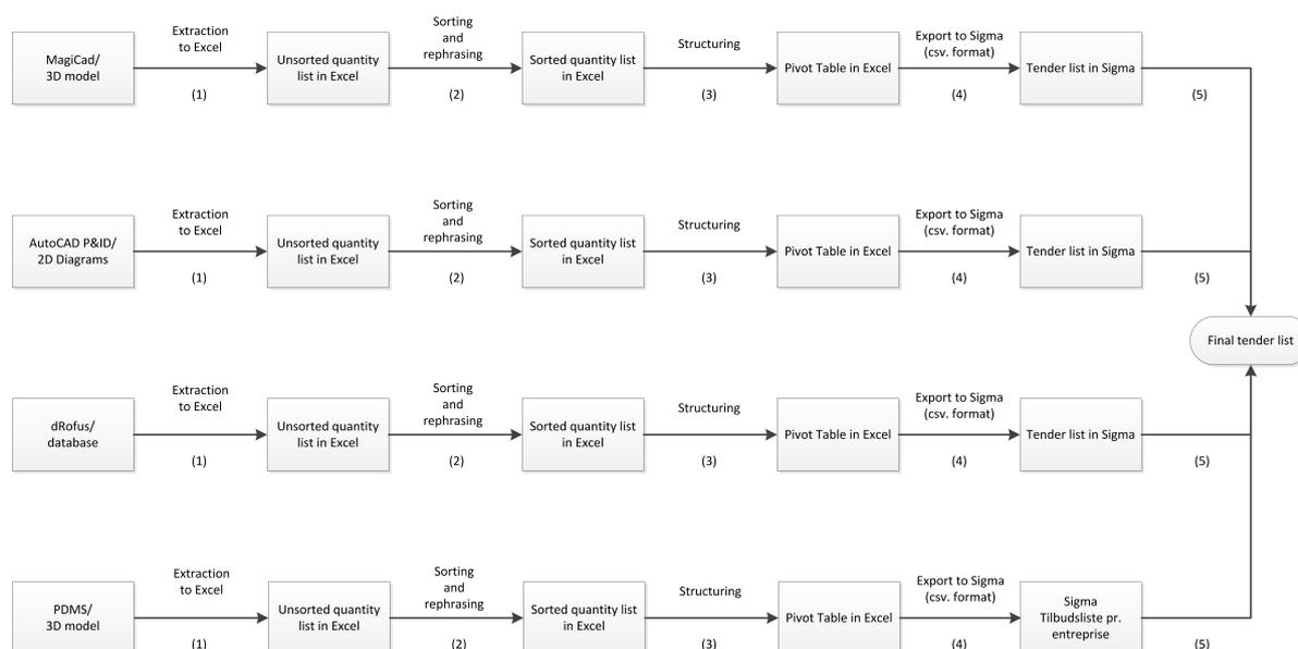
**Figure 6.12:** Measurement of digital quantities in the MB project (also shown in Appendix C)
