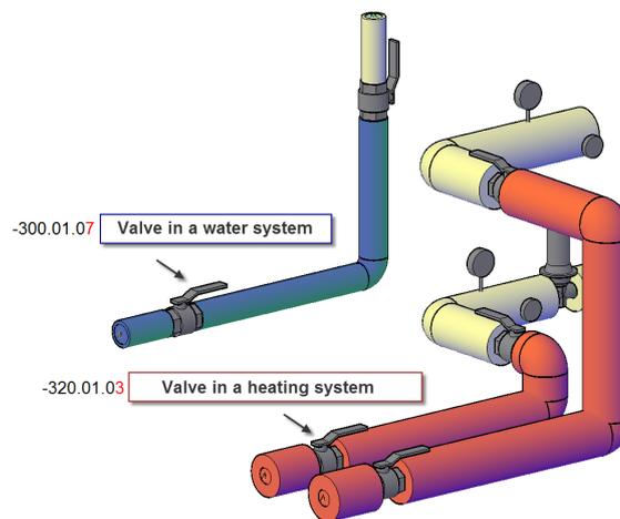
**Figure 6.3:** Comparison of valve in different systems [Karved (2009)]
