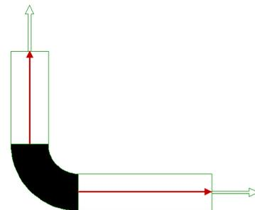
**Figure 6.19:** Measurement rules for ducts/pipes (MB) corresponding to measurement rule (c)
