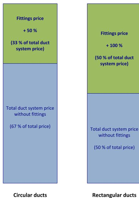
**Figure 6.8:** Price impact of fittings for ventilation on the TechFac project [Freddi Lading (Brøndum)]
