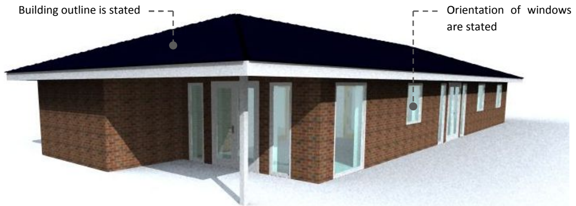
Figure 33 Rendering of the south-west and north-west facing facades from the BIM-model (Level 1.0). At this point, the BIM-model contains information of the building outline and the orientation of windows.
