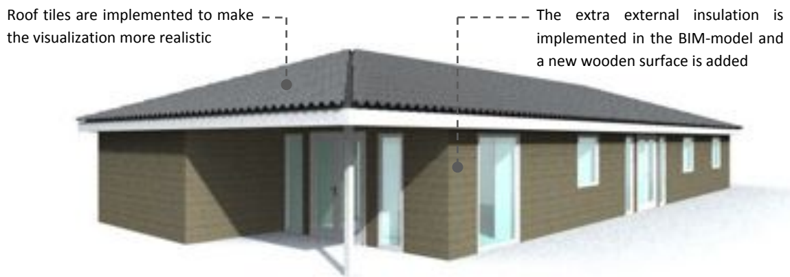
Figure 37 Rendering of the south-west and north-west facing facades from the BIM-model (Level 1.2)
