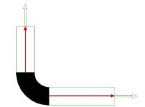
**Figure 6.18:** Measurement rules for ducts/pipes (TechFac) corresponding to measurement rule (b)
