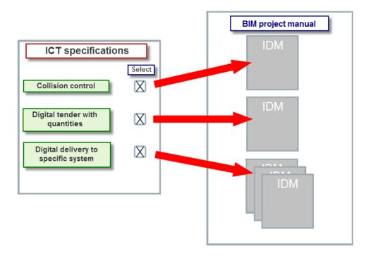
Figure 4.5: ICT specification in relation to IDM [Hejnfelt (2011)]
