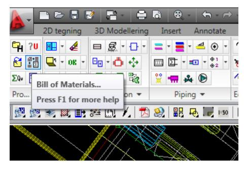
In there it possible to set up a **selection set**, which corresponds to the wanted trade contract. In this case **Ventilation** was choosed. This **selection set** can be assigned to all the relevant **model drawings** and simultaneously assign the wanted **systems**. To be on the safe side all **systems** can be choosen, but
