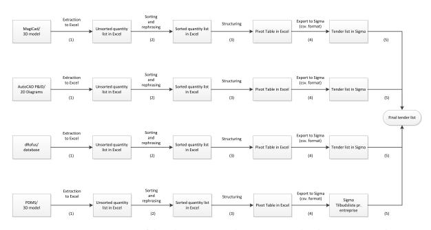
Figure 6.12: Measurement of digital quantities in the MB project (also shown in Appendix C)
