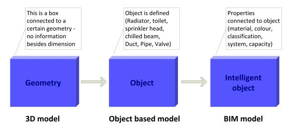
Figure 2.3: Illustrations of the the different digital building models
