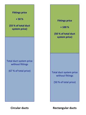
Figure 6.8: Price impact of fittings for ventilation on the TechFac project [Freddi Lading (Brøndum)]
