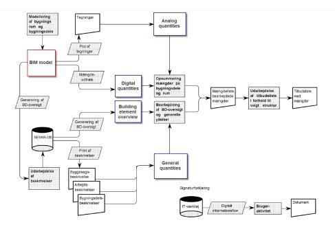
Figure 6.11: Extracting quantites - digital and analog process (Bips F110a, 2008)
