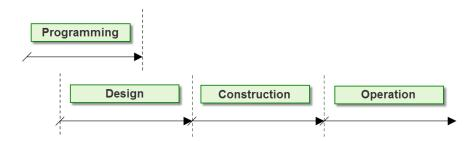
Figure 3.2: Illustration of the DBB contract form [Anlaegsforeningen (2011)]
