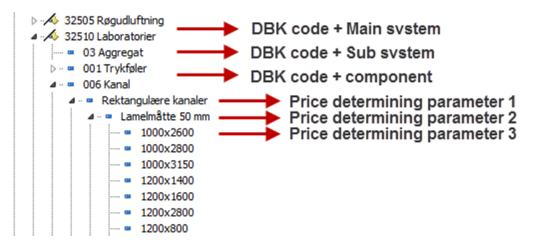
Figure 7.3: Structure of tender list for the MB project
