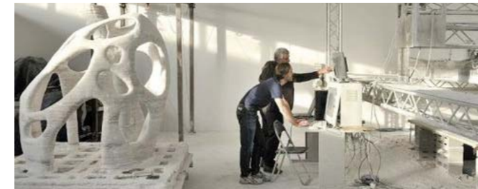
Enrico Dini prints large scale cement based structures
