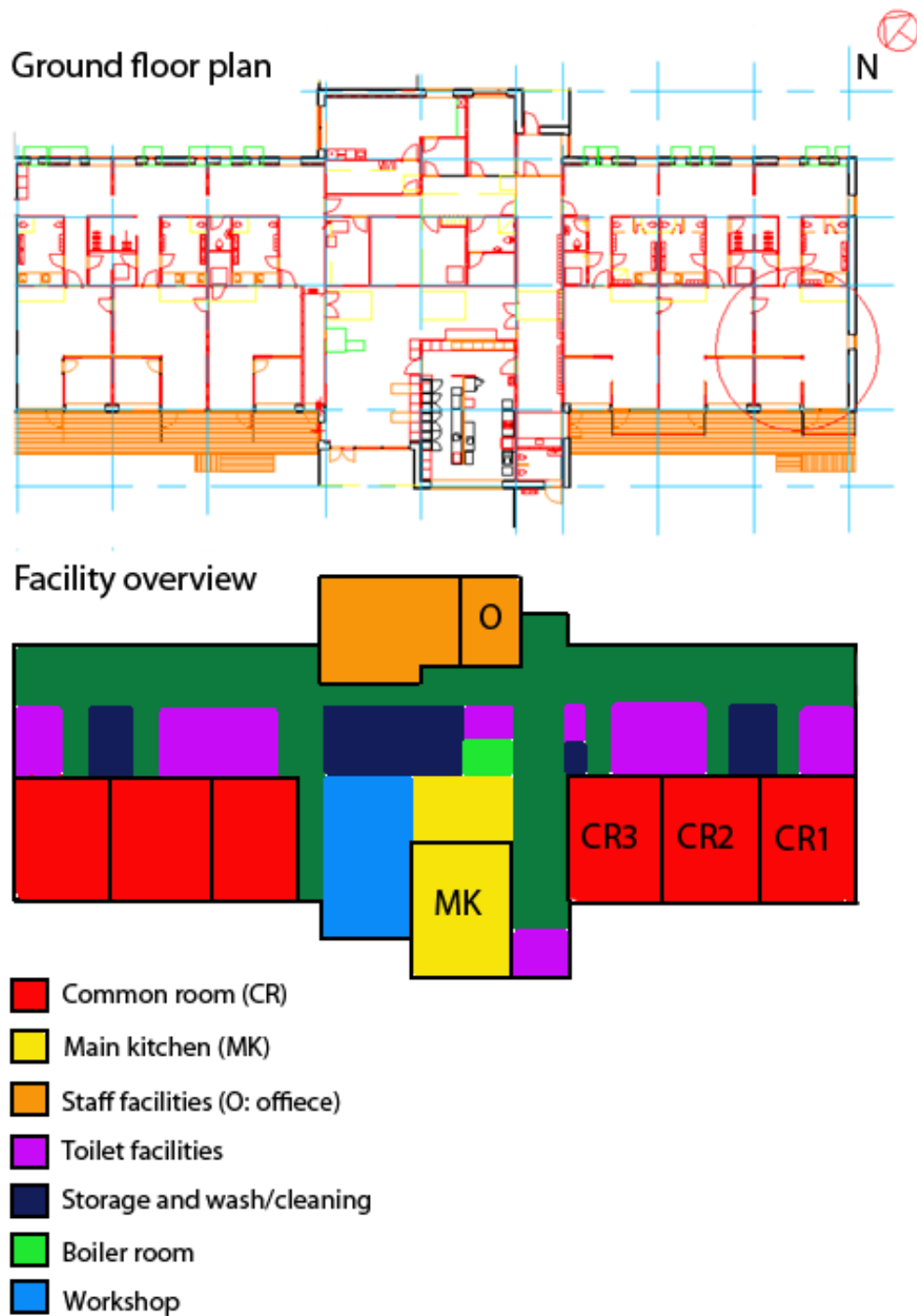
Figure 2.4- Top: ground floor plan of Tranehavevej daycare institution; Bottom: facility overview, the two common rooms (CR1 and CR2) are for kindergarten kids and CR3 is for nursery kids.
